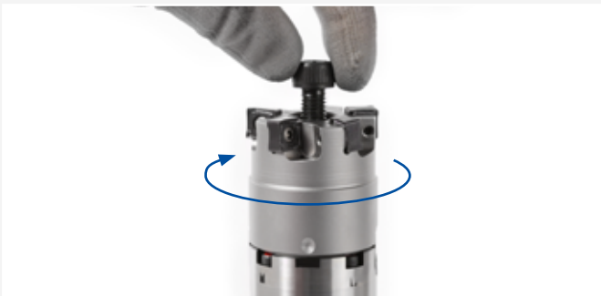
4. Lightly screw the milling cutter clamping screw into the thread bore of the milling cutter arbor by hand.
