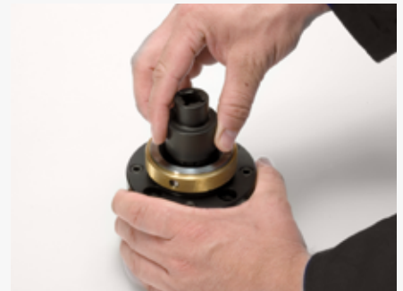
3. Turn clockwise until the lug on the clamping cartridge engages with the clamping pin.
