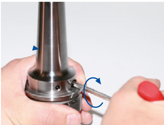
Figure 2: Tighten the clamping screw and observe the minimum revolutions
