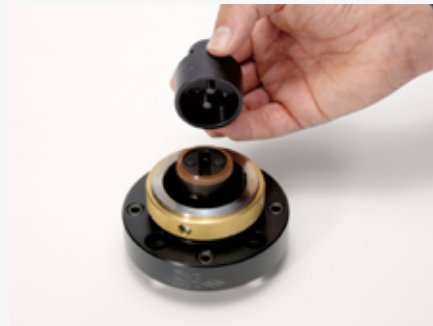
2. Fit socket to the clamping cartridge.
